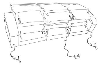
① Make sure all plugs are connected on the product before plugging the power cords into a wall outlet otherwise product damage may occur. The USB ports (where applicable) are designed with working voltage of 5V and can NOT be used to supply power for laptop computers (neither PC or Mac). Plugging a laptop computer to the USB port may end up damaging either the computer or the USB port due to unmatched working voltage.
